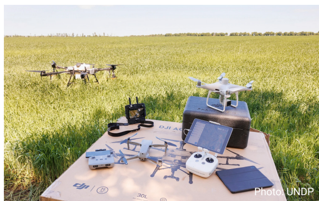
Agricultural drones sprinkle on average up to 40% less active substance (herbicides dissolved in water) allowing more uniform and more accurate spraying.
